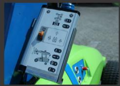
Multifunction control panel in operatorfriendly design with integrated buttons and signal lights, Double action safety keys and Gyro functionality are both in the standard setup on the Winlet 575.
